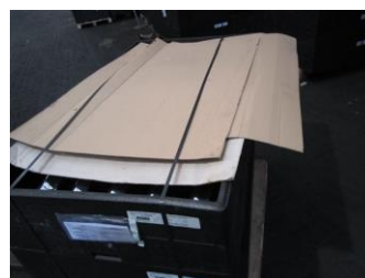
Missing pallet end cap
